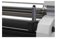
> Adjustable stopper to assist with cone rolling.
